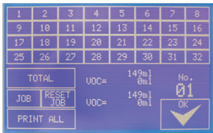
Consumption of up to 32 colours/materials (resin, catalyst and solvent) can be independently monitored for VOC content and material usage.
