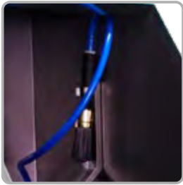
Brush with water for cleaning the exterior of the gun
