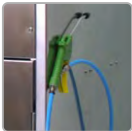
Gun with coupling for cleaning interior areas
