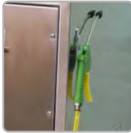
Gun with coupling to clean interior areas
