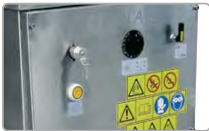
Opening handle, on/off and timer on the front door.
