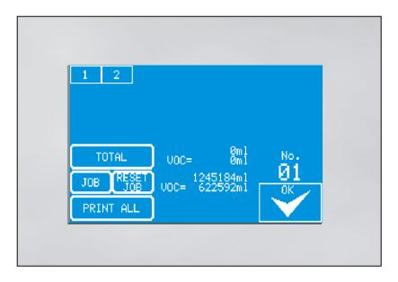
Use the keys [1] and [2] to select the valve, respectively the component of which you wish to read the consumption.
