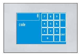
The value to be set is shown at the upper part on the left side. The value will be deleted by pressing the "DEL" key (one decimal place each per key depression). The value will be entered into the system by pressing the number fields and by pressing the field "ENT".
