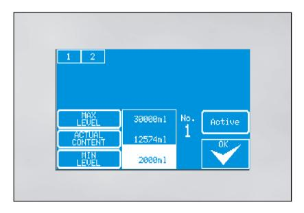
The integrated container control serves the control of the container level without additional sensory mechanism. If a container shall be controlled, it is necessary to deposit into the menu its filling level prior to use.
