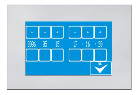
Press the key [SET CLOCK] in order to set the internal clock of the system. The clock has a movement reserve of approximately 10 - 14 days. The clock is necessary to print reports and to store alarm messages.
