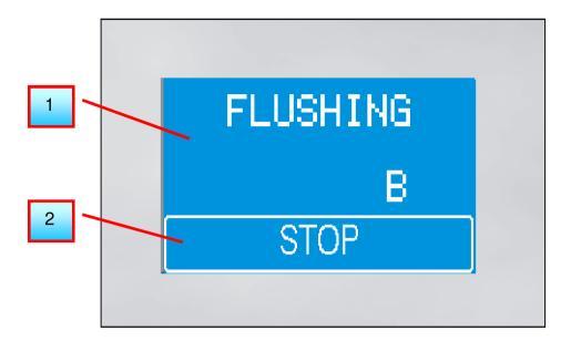
[1] Alternating side "A" and side "B" are being displayed. If an automatic mixer head has been connected, the two flushing valves will open according to the display. If you have manual mixer heads with ball valves, the display will be of help to remind you to clean the two ball valves
