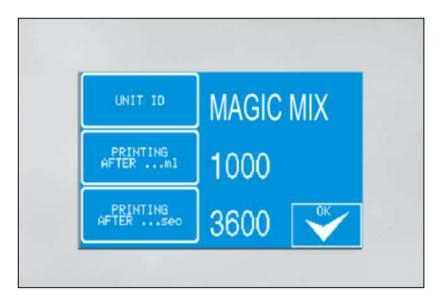
[UNIT ID] displays the name of the mixing system which appears on the prints. It is, therefore, possible to distinguish between the prints of different systems. The name can have up to 10 characters.
