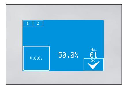
With the keys [1] and [2] you can chose the valve, respectively the component in order to set the VOC-value.
