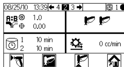
FIG. 17. Run Mix Spray (Screen 2)
