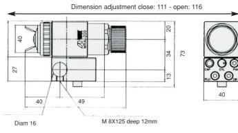
Nipples 1/8" F. Fixing hole M8X1.25
