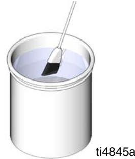
FIG. 14: Use solvent-dipped soft-bristle brush
