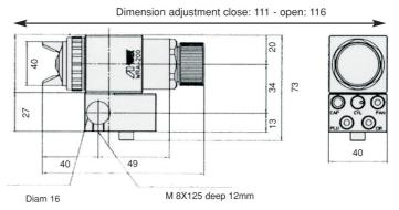
Nipples 1/8" F. Fixing hole M8X1.25
